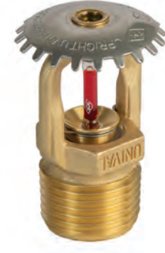
UV311 Dik Tip Sprinkler Hızlı Tepkili, Pirinç Upright, Quick Response, Brass K5.6 - 1/2" - 68C, 79C, 93C, 141C
