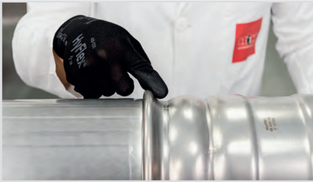
Oversize preslemenin görsel incelemesi Visual inspection of oversize pressing
