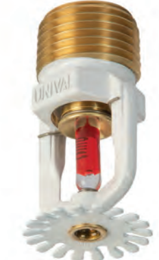
UV320 Sarkık Tip Sprinkler Hızlı Tepkili, Beyaz Pendant, Quick Response, White K5.6 - 1/2" - 68C, 79C, 93C, 141C
