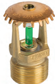
UV410 Dik Tip Sprinkler Standart Tepkili, Pirinç Upright, Standart Response, Brass K8.0 - 3/4" - 68C, 79C, 93C, 141C
