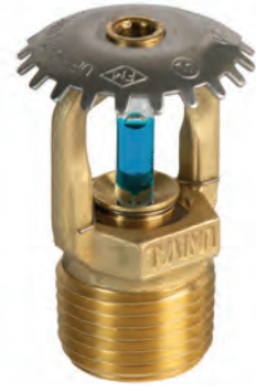
UV310 Dik Tip Sprinkler Standart Tepkili, Pirinç Upright, Standart Response, Brass K5.6 - 1/2" - 68C, 79C, 93C, 141C
