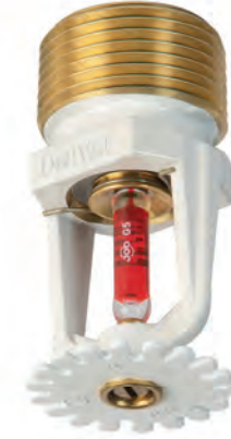
UV420 Sarkık Tip Sprinkler Hızlı Tepkili, Beyaz Pendant, Quick Response, White K8.0 - 3/4" - 68C, 79C, 93C, 141C
