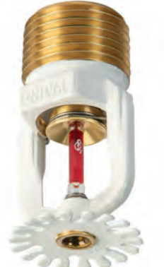
UV321 Sarkık Tip Sprinkler Hızlı Tepkili, Beyaz Pendant, Quick Response, White K5.6 - 1/2" - 68C, 79C, 93C, 141C
