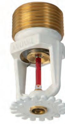
UV421 Sarkık Tip Sprinkler Hızlı Tepkili, Beyaz Pendant, Quick Response, White K8.0 - 3/4" - 68C, 79C, 93C, 141C
