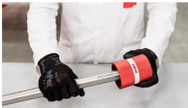
Figure 26 - Deburring the pipe
