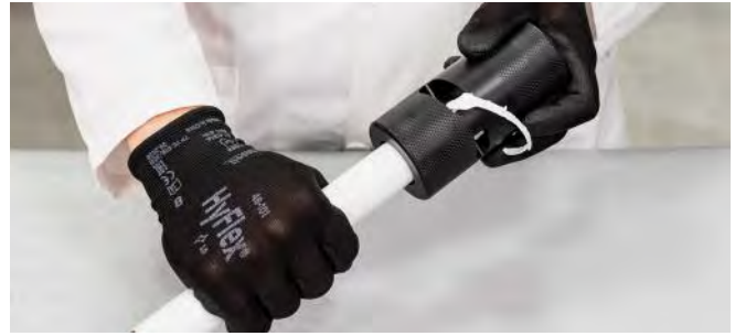
Figure 29 - Stripping (steelPRES PP coated)
