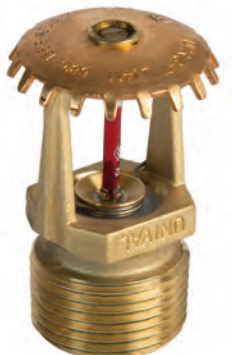
UV411 Dik Tip Sprinkler Standart Tepkili, Pirinç Upright, Standart Response, Brass K8.0 - 3/4" - 68C, 79C, 93C, 141C
