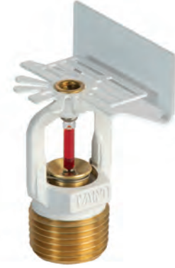
UV341 Duvar Tipi Sprinkler Beyaz Standart Tepkili Horizontal Sidewall White Standart Response K5.6 - 1/2" - 68C, 79C, 93C, 141C
