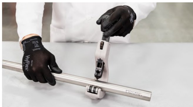
Figure 25 - Cutting the pipe to length
