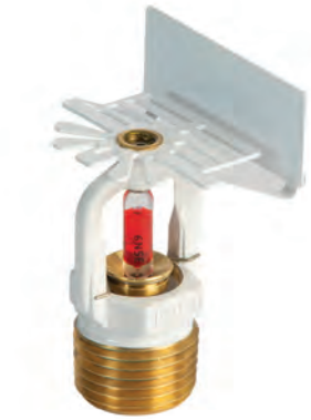
UV340 Duvar Tipi Sprinkler Beyaz Standart Tepkili Horizontal Sidewall White Standart Response K5.6 - 1/2" - 68C, 79C, 93C, 141C
