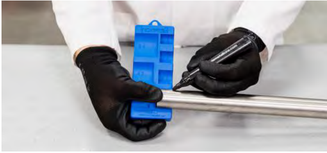
Figure 28 - Marking the insertion depth
